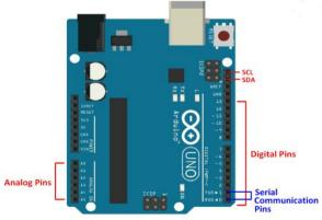
Fig.3 Arduino UNO board
