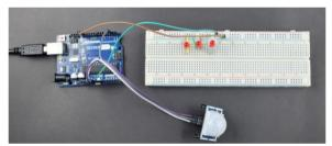
Fig.5 Connections on the breadboard
