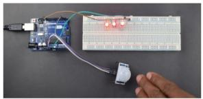
Fig.9 LEDs glowing when the motion is detected
